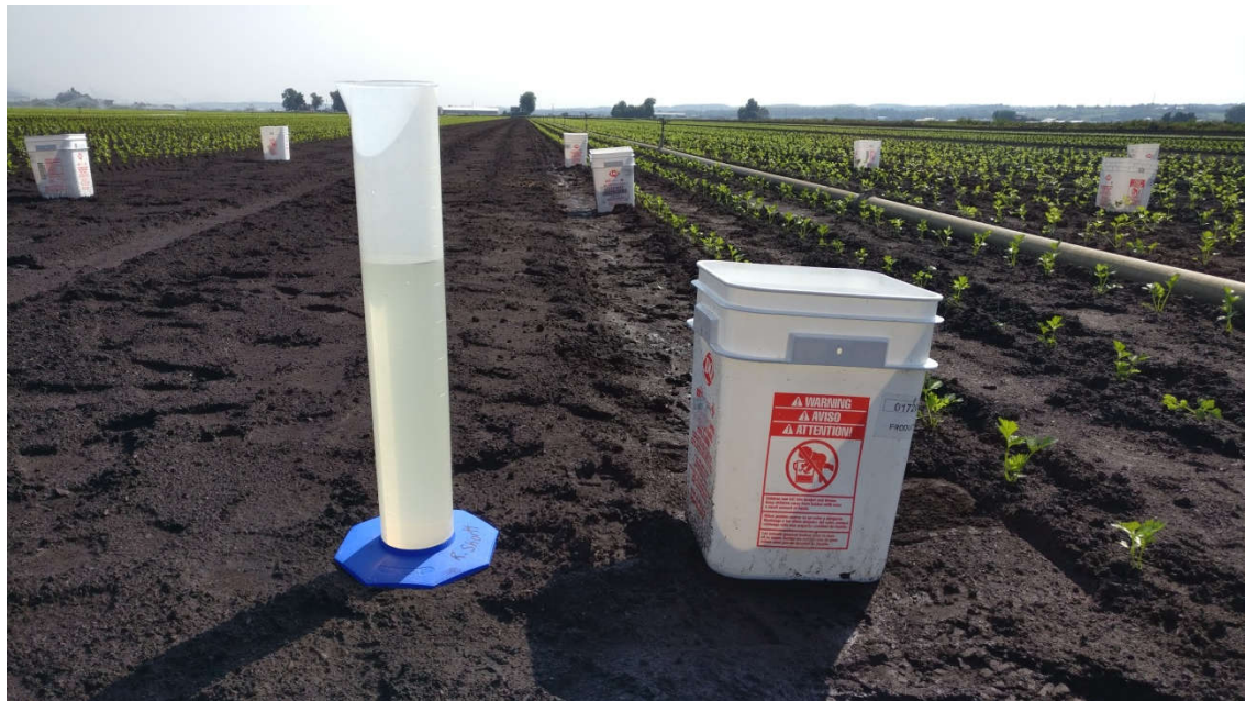
Figure 5: Example of Measuring Catch Can Intercepted Water
